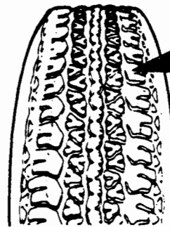
EDGE OF TREAD BLOCKS WORN
