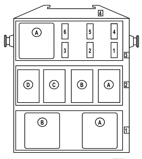
Allocation of fuses and relays (according to equipment level)
