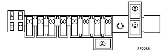
Allocation of fuses and relays (according to equipment level)
