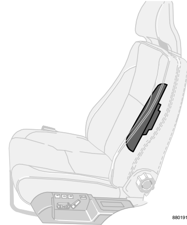
The side impact airbags are installed in the front seat backrest frames
