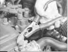
Connect the other end of the black jump lead to a bolt or bracket on the engine block, well away from the battery, on the vehicle to be started.
