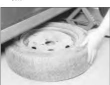
6 Temporarily place the spare wheel under the sill as a precaution should the jack topple.
