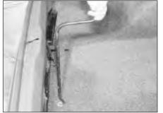
1 In the boot, use the wheel brace to loosen the spare wheel cradle bolt.
