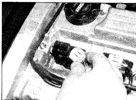
18.8 Disconnect the wiring plug from each coil
