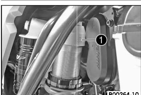
The shock absorber part number ① is stamped on the top of the shock absorber above the adjusting ring on the engine side.
