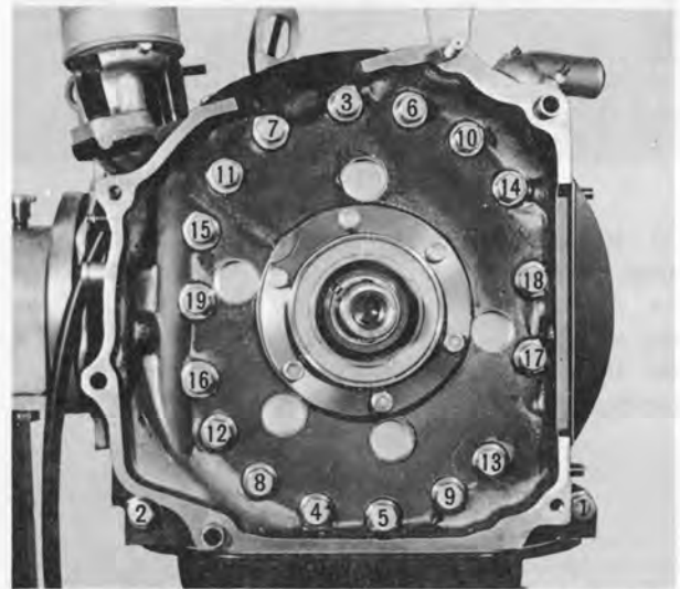
Fig. 1-17 Tension bolts loosening order
