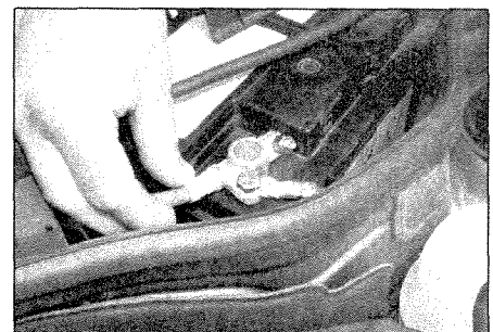
4 Check the security and condition of the battery connections.
