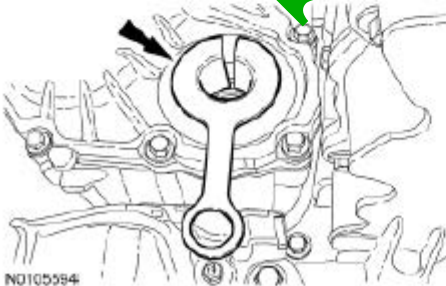
Fig. 31: Inserting Seal Protector Into PTU Deflector ID Courtesy of FORD MOTOR CO.
