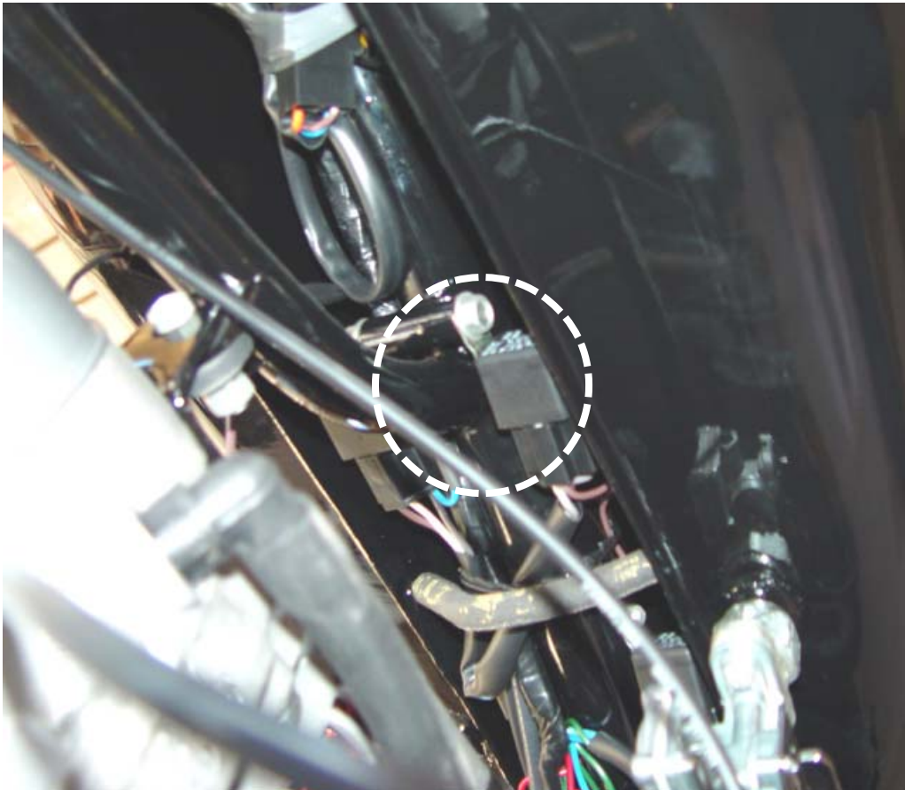
The headlight relays are located under the fuel tank
