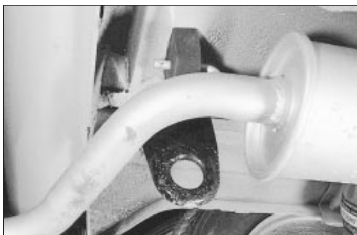
Rear lashing eye - not to be used for towing
