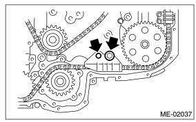
(6) Install the chain tensioner lever (LH).
