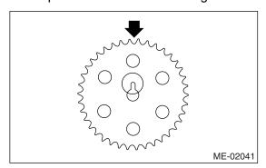
4) Align the intake cam sprocket as shown in the figure.
