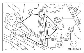
(8) Check that each mark on the sprocket and timing chain is matched, and then draw out the stopper pin from chain tensioner.
