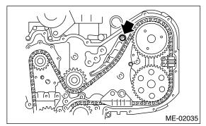
10) Remove the chain guide (LH: between cams).
