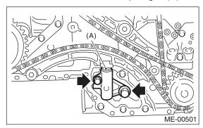
4) Remove the chain guide (RH: between cams).
