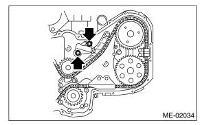
9) Remove the chain tensioner lever (LH).
