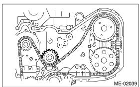
(4) Install the chain guide (LH: between cams).
