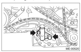
(7) Adjust the clearance between chain guide (RH) and chain guide (center) within 8.4-8.6 mm (0.331 — 0.339 in). Install the chain guide (center).
