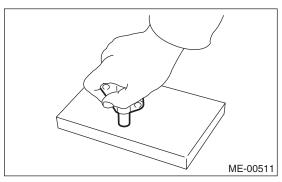
2) Using the ST, align the "Top mark" on crank sprocket to 9 o'clock position as shown in the figure ST 18252AA000 CRANKSHAFT SOCKET
