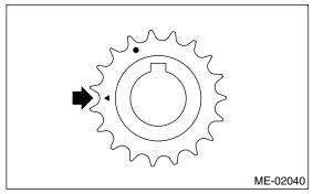
3) Align the key groove on exhaust cam sprocket to 12 o'clock position as shown in the figure.
