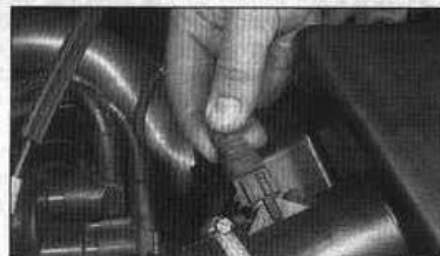
C Check the mass air flow sensor or inlet air temperature sensor wiring connector for security.
