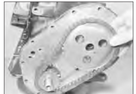
14.11 Removing the sprockets and timing chain
