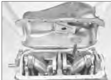
11.9 Refitting the sump
