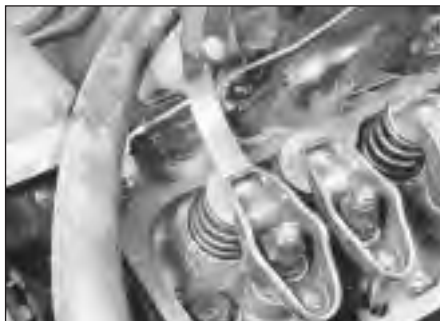
7.10 Checking a valve clearance
