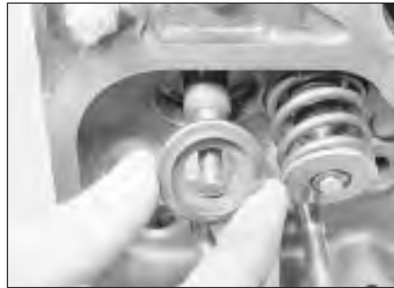
9.17 Fitting an exhaust valve rotator
