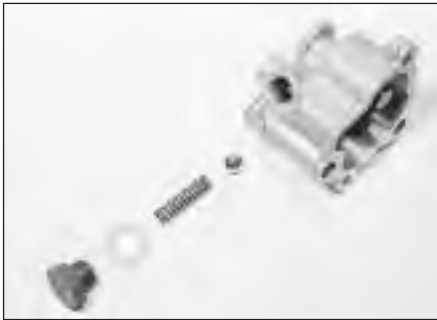
13.4 Oil pump and pressure relief valve components
