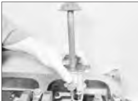
12.2b . . . and remove the oil pump
