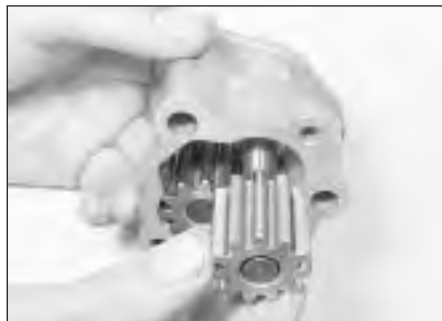
13.3a Removing the oil pump driving gear . . .
