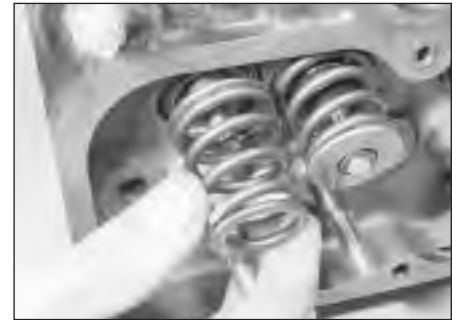
9.18a Fit the valve spring . . .
