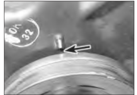
7.7 Ignition timing marks (arrowed) in alignment
