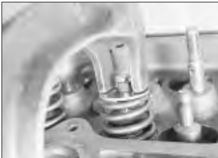
9.20 Compress the spring and fit the collets
