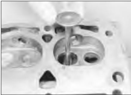
9.15 Fitting a valve to its guide
