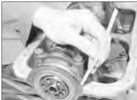
11.7 Insert the cork strips in the main bearing cap grooves
