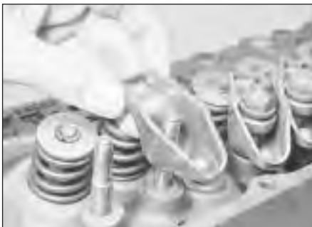
9.24a Fitting a rocker arm . . .
