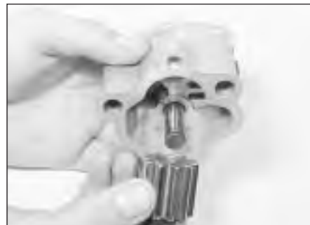
13.3b . . . and the driven gear
